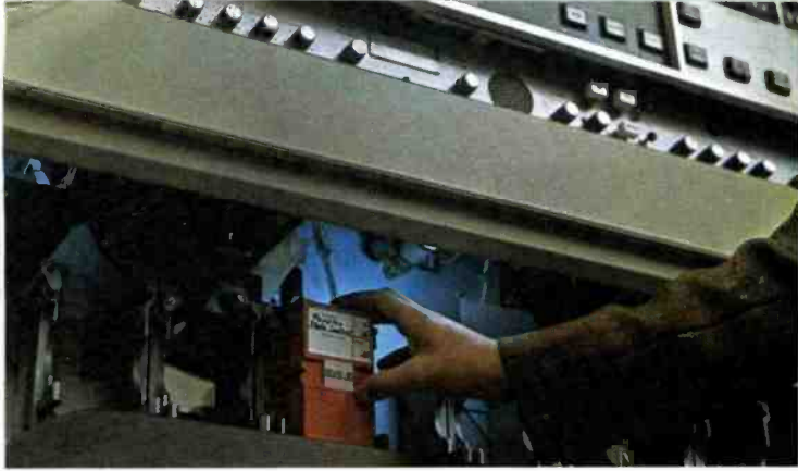
EASY TO LOAD, as many as 22 cartridges can be stored in the magazine.
