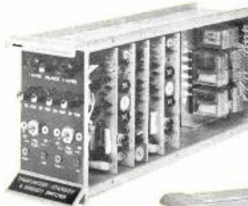
ACCESSORY NEST, consisting of slide-in modules in rack mounting frame.
