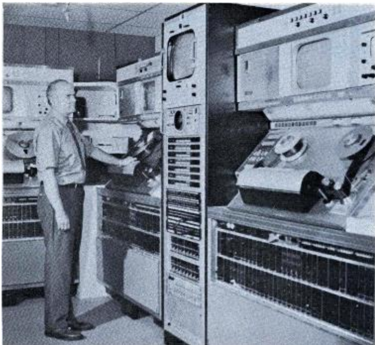
TELECINE area includes three TR-70 tape recorders which share both production and playback duties.
