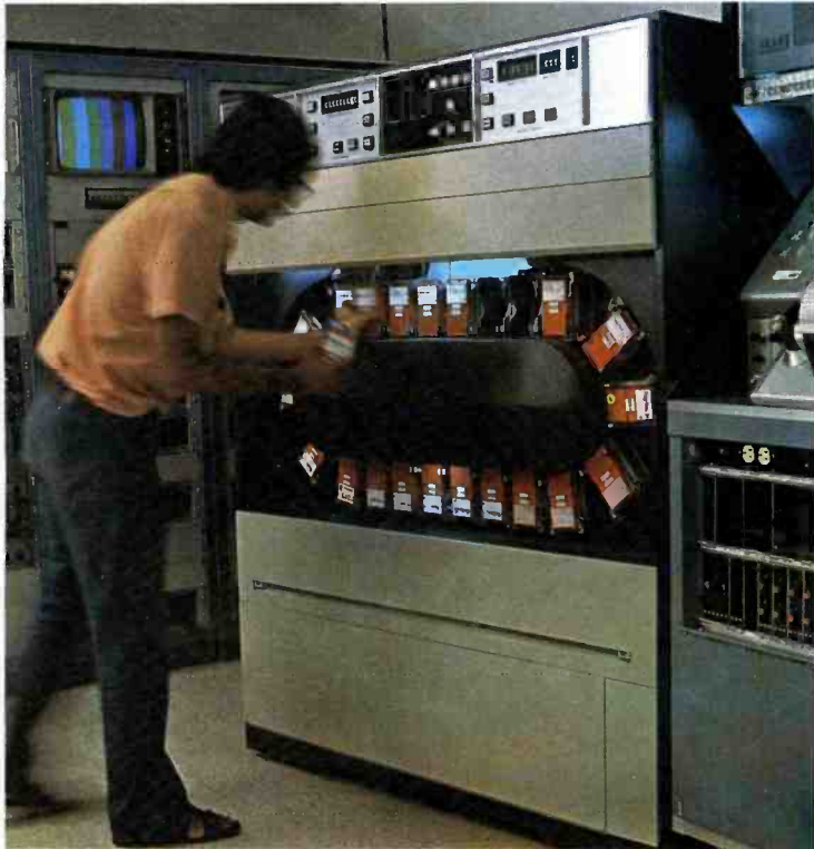
LAST MINUTE CHANGE from traffic is handled easily. Cartridges are exchanged and the new commercial is ready to play.
